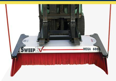
The Megamax forklift sweeper combines all the characteristics of the heavy duty Megasweep forklift sweeper, but with added side retainers, which will hold bulk volumes of material in front of the brush without spillage.
