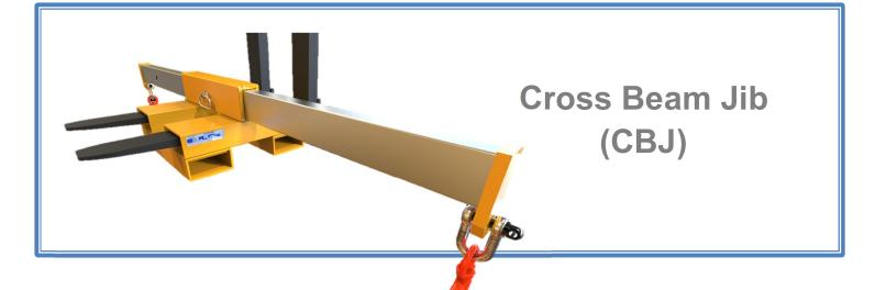
The Cross Beam Jib offers the flexibility tohandle loads via a traditional jib method or via a spreader beam all in one attachment. Simply remove the retaining pin from the beam and slide into the desired position, then replace the pin, ensuring the beam is locked in that position. Then simply drive slowly dorwards until the truck forks are located in the attachment sleeves and simply use the retaining chain to fix the attachment to the forktruck. Then lifting can occur.
