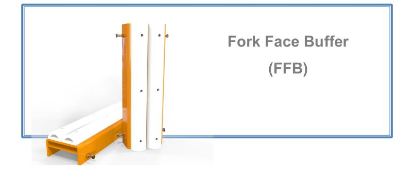
The fork face buffer is a retro-fitted safety device for use with any size fork section. The buffers consist of a mild steel pressed section with a plasticised foam buffer bonded to the front face to ensure delicate and fragile loads are kept clear of carriage and fork shank contact. The buffer is retained via four securing screw pins to ensure an even and safe fitment to the fork shank, as well as easy and quick removal when lifting is complete
