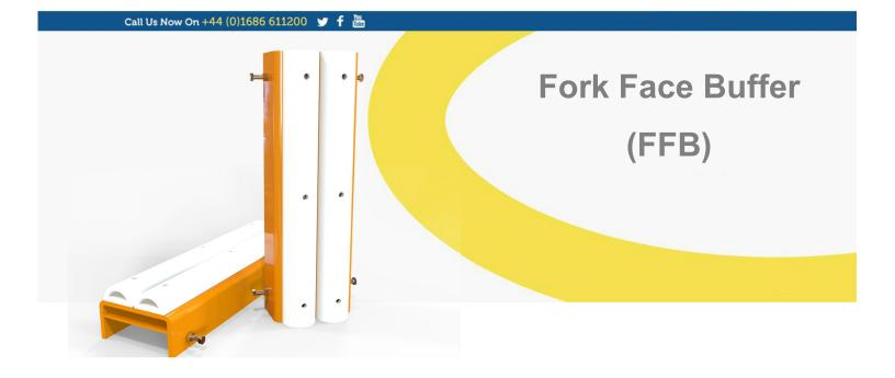
The fork face buffer is a retro-fitted safety device for use with any size fork section. The buffers consist of a mild steel pressed section with a plasticised foam buffer bonded to the front face to ensure delicate and fragile loads are kept clear of carriage and fork shank contact. The buffer is retained via four securing screw pins to ensure an even and safe fitment to the fork shank, as well as easy and quick removal when lifting is complete
