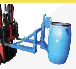
Designed for handling open top plastic Mauser (egg-shaped) drums, this rim grip drum handler comes fitted with a gripping head that allows the drums to be picked up via the drum lip.
