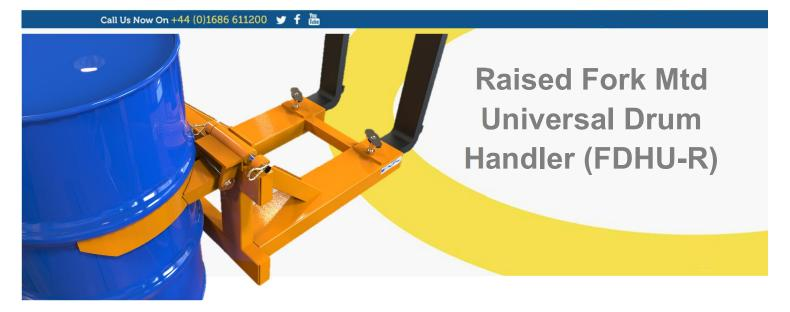
Our best selling drum handler has a fully automatic action. The attachment has two curved arms which hinge at one end. To lift a drum, approach it with the clamp arms horizontal and postioned halfway up the drum, between two rolling hoops. When the arms contact the drum they will open automatically, falling back around the drum as you proceed forwards. When the attachment is raised the arms will grip the drum tightly under the upper rolling hoop.
