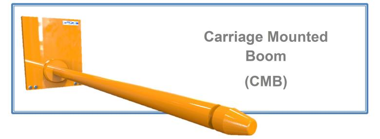
Carriage mounted booms are ideal for handling cylindrical obects with a hollow core, such as rolls, reels and carpets. The unit comes complete with a solid steel lifting tine, manufactured to a specific length to suit your roll length and material type. Our carriage mounted booms comes as standard with heavy duty machined rear hangers for connecting to the truck carriage. Quick release hangers can also be fitted upon request.
