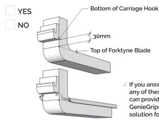
TYPE B - is there 20mm clearance between the side of the Carriage Hook and the side of the Forktyne Blade?
