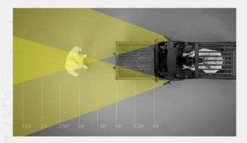
GenieGrips® Loading Mirrors are a forward view mirror system designed for forklifts.
