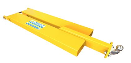
Our forklift hitch enhances conventional forklift capabilities, allowing for effortless moving of objects like trailers with precision.
