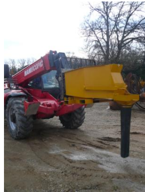
BSB skip fitted with a 1 meter long hose
