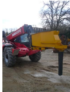
BSB skip fitted with a 1 meter long hose
