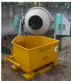
BSB skip filled from a site concrete mixer
